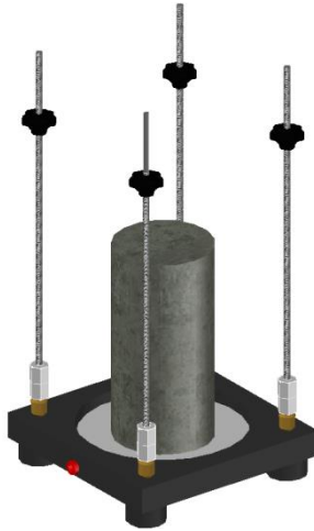
Figure 9. Place the concrete sample over the sponge
