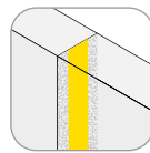
Controlled crack joint
