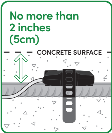
4 Install the transmitter on rebar no more than 2 inches (5cm) from concrete surface
