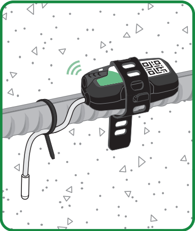
7 Pour concrete and monitor results in the mobile app or remotely with SmartHub™
